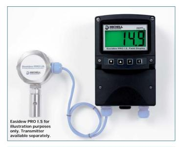
The Intrinsically Safe Field Display is a 4-digit loop-powered local monitor for the Easidew PRO I.S. and Easidew I.S. transmitters. It is certified with ATEX, IECEx, and FM and housed in an IP66 enclosure with a terminal compartment for wiring. The measurement unit can be labelled as ppm, ppm, °C dp or °F dp.
