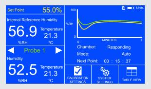
A 4.3" LCD touch-screen runs a powerful UI, which displays all measured values from the reference and probes under test, along with a graphical trend indication of chamber stability. It is also capable of automating complete validation procedures with ease, and providing a complete logged output in csv format straight to your USB memory device, to minimize the time you spend taking readings.
